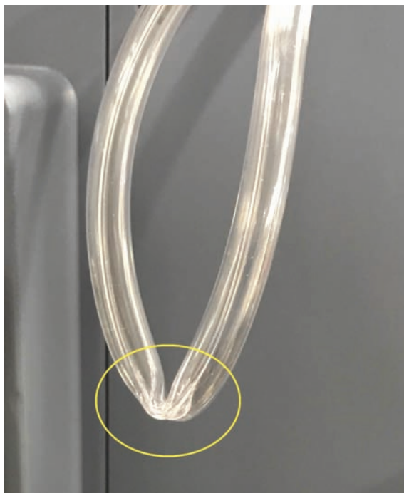
Figure 4. Kinked oxygen tube.
