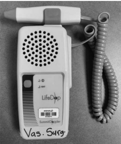
Figure 1. Five- to 10-MHz continuous wave Doppler.
