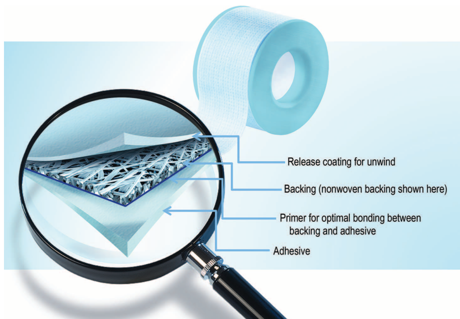
FIGURE 1. Anatomy of medical adhesive tape.
